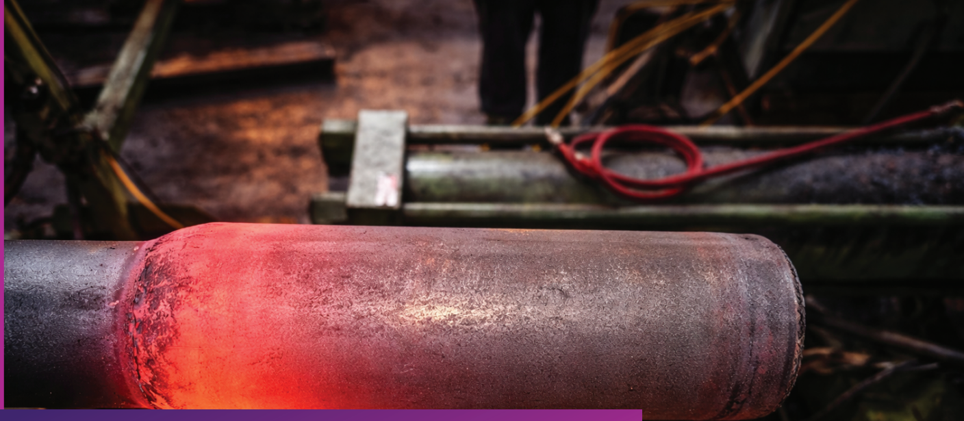
SECTION OF UPSETTED PIPE
